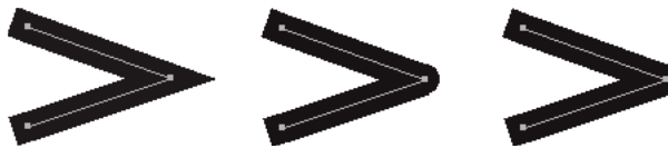
Miter, round, and bevel joins.
