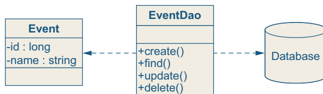
Figure 7.1 A diagram of Event and EventDao as they interact with the database
